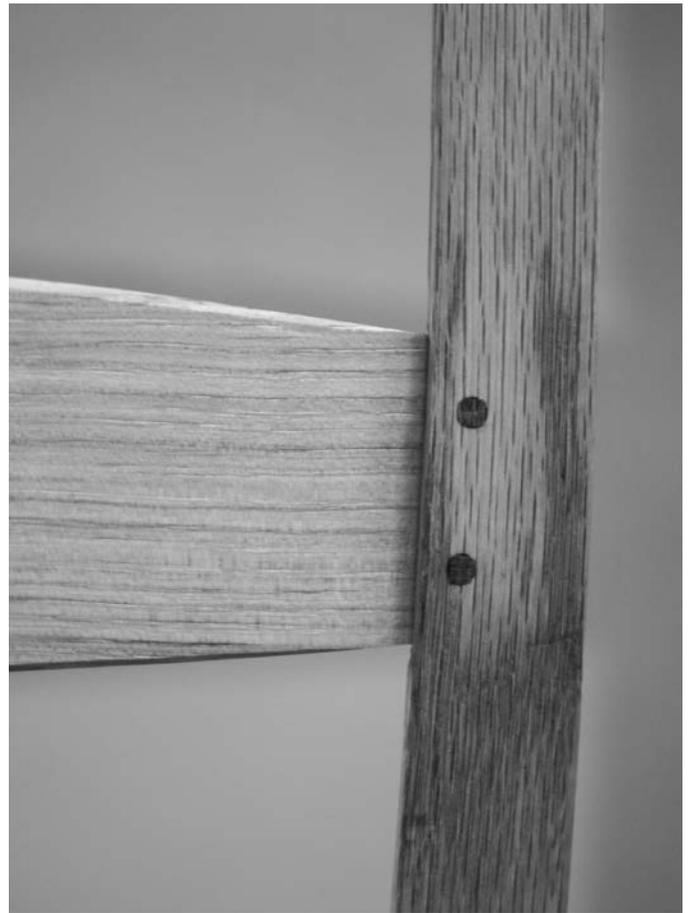
*Figure 3. A detail of the lower slat and the pegs that hold it in place.*
